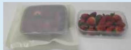
Figure 1. The packed strawberries in EcoBioCAP packaging (left) and the selected benchmark packaging (right). (Photo from MS19) >>>>>
